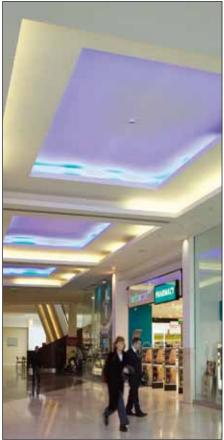
Gillespie's highly flexible Zerodec laminated GRG facilitated the production of the striking contemporary forms that make up the interior design, with the medium allowing prefabrication of the ceiling and atria mouldings off-site to sculpt the natural and artificial light features. The curved and elliptical profile sections were modelled in CAD and moulded at the company's factory in Surrey before being transported to site for the final precision fitting and finishing stages.
